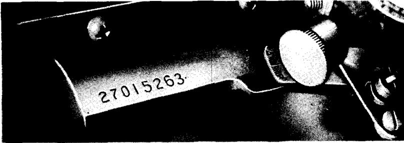
ENGINE SERIAL NUMBER—ON RIGHT SIDE OF BLOCK
