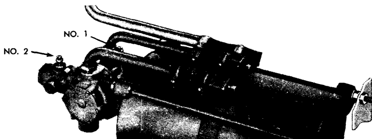
HYDROVAC BLEEDING POINTS AND SEQUENCE
