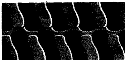
ONE TYPE NON-DIRECTIONAL TREAD PATTERN
